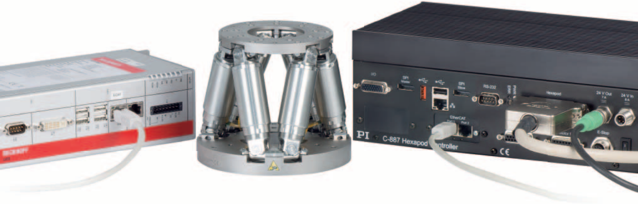
Example configuration: H811 miniature hexapod with C-887532 motion controller with EtherCAT interface and motion stop. The EtherCAT master, here a Beckhoff controller, is provided and programmed by the customer.
