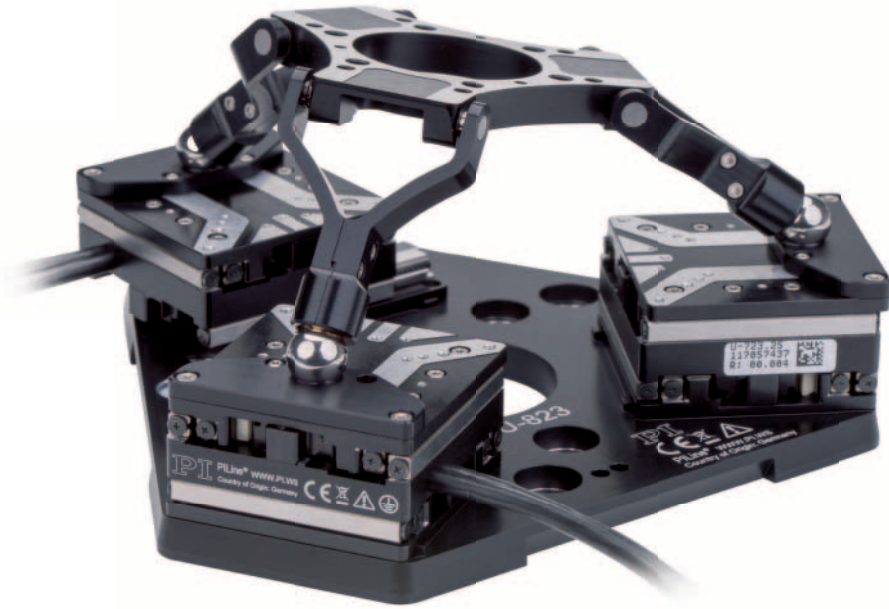
This miniature hexapod was developed on the basis of fast PILINE® ultrasonic motors to enable fast motion in all six spatial directions (three linear, three rotational). The parallel-kinematic SpaceFAB design makes a particularly low overall height of only 80 mm possible. The individual axes can be commanded with up to 120 mm/s.
